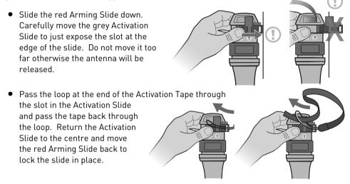
Take the lifejacket Fixing Buckle (Supplied) and pass the tape through the slots as shown below, making sure that tape does not get twisted.
